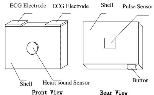
Figure 2. Integrated structure figure of acquisition unit
