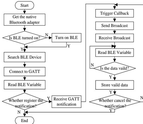
Figure 5. BLE communication and data storage flow chart
